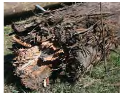
The EF3 tornado twisted this pole near Mapleton and snapped it off.
